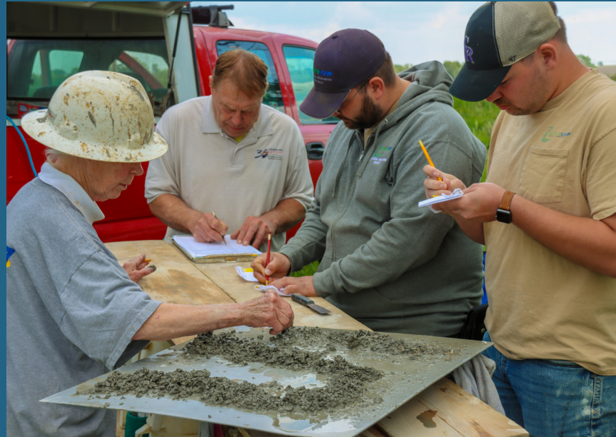
The 2025 Lower Loup NRD field season included technicians working with UNL Hydro-geologist Susan Lackey on test holes drilled north of Fullerton. The holes were drilled at the base of the aquifer as research in response to well interference issues in an area with little saturated thickness.
