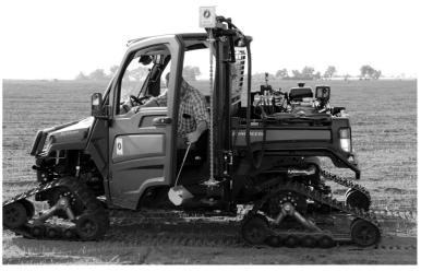
Funding from a Nebraska Environmental Trust (NET) Grant assisted in the purchase of a UTV and soil sampling probe for deep soil sampling. The UENRD is soil sampling in the Phase III areas of the district to see how much residual nitrogen is being left in the soil.
