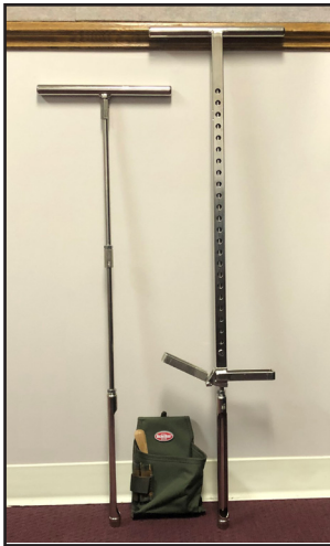
Left: Collapsible Sampler Right: Backsaver Sampler
