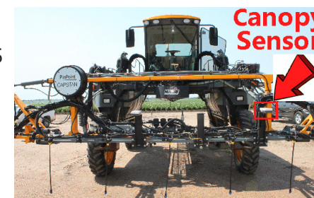
Project's high clearance applicator equipped with OptRx Canopy Sensor.
